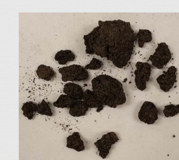
Figure 7: Granulated soil/biochar pellets 4 (5:1 ratio)
