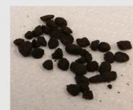
Figure 4: Pellets sample #1 with soil 1/biochar (10:1 ratio)
