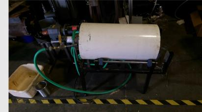
Figure 2: Granulator used to make soil/biochar pellets
