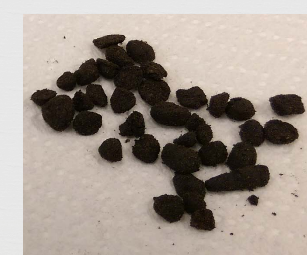
Figure 4: Pellets sample #1 with soil 1/biochar (10:1 ratio)
