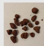
Figure 5: Pellets sample #2 with soil 3/biochar (10:1 ratio)
