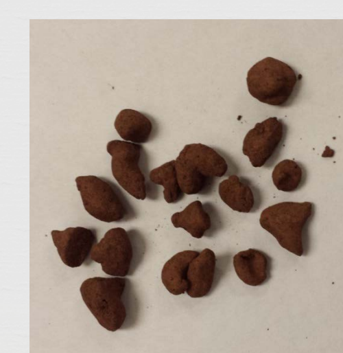
Figure 5: Pellets sample #2 with soil 3/biochar (10:1 ratio)
