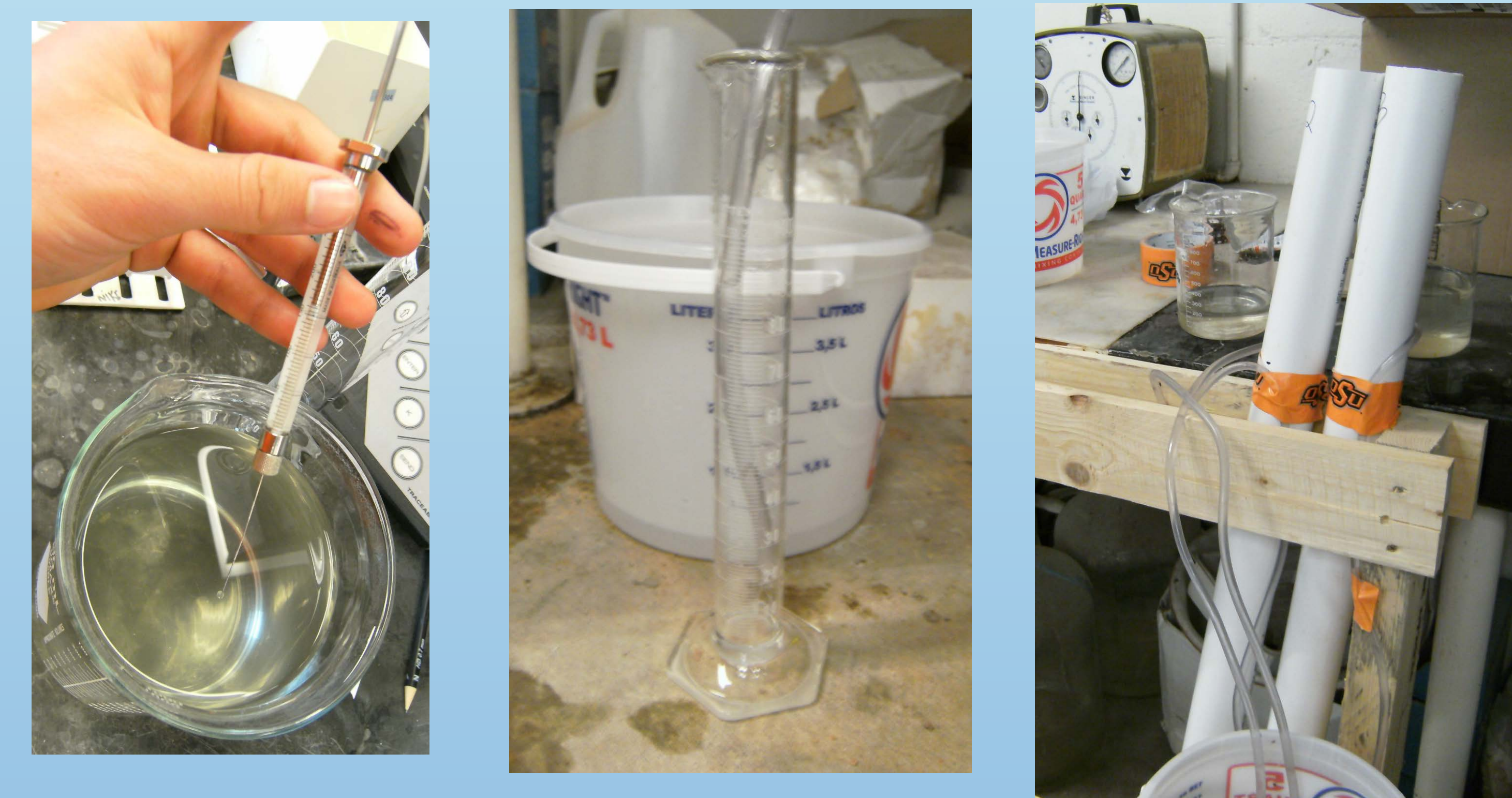
From left to right: preparing the bacteria mixture, measuring flow rate, biosand filter setup
